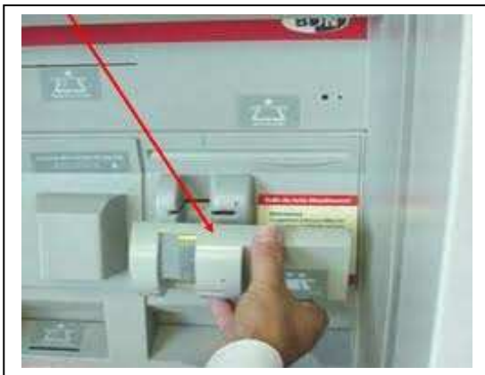
SKIMMER BEING FIXED IN THE ATM MACHINE
